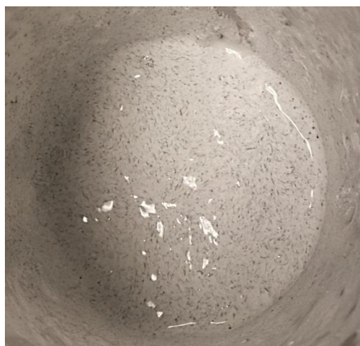
Figure 2.2. Paste with titanium fibers distributed in bioglass
